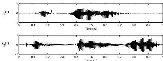
Figure 3: The source signals: each signal was spoken by a different male and recorded with sampling rate of 16kHz.  $s_1(t)$  is a recorded word of “good morning” and  $s_2(t)$  is a Japanese word “konbanwa” which means “good evening”.
