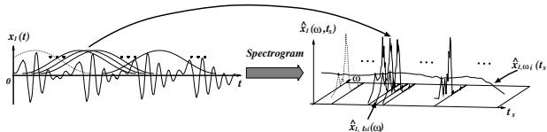
Figure 1: Windowed-Fourier transform (spectrogram)
