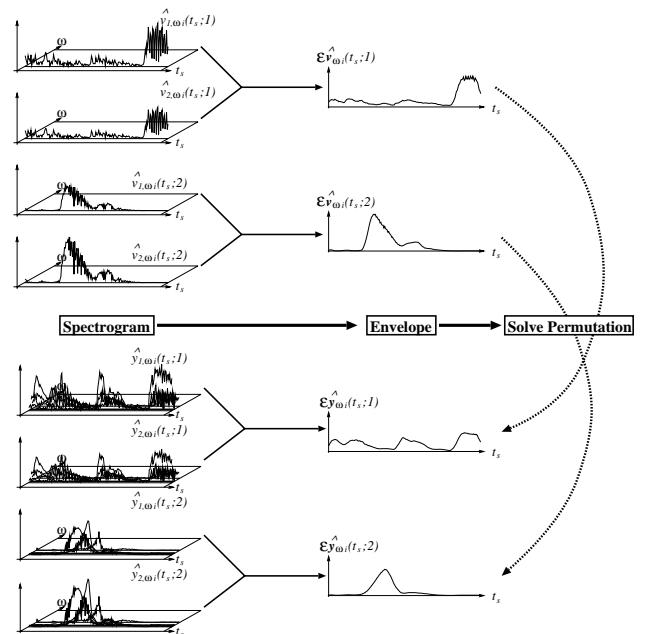
Figure 2: Construct separated spectrogram
