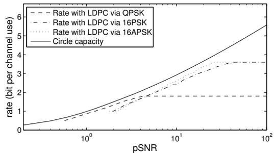
Fig. 7. Achievable rates with QPSK, 16PSK, and 16APSK compared with capacity under circular constraint.
