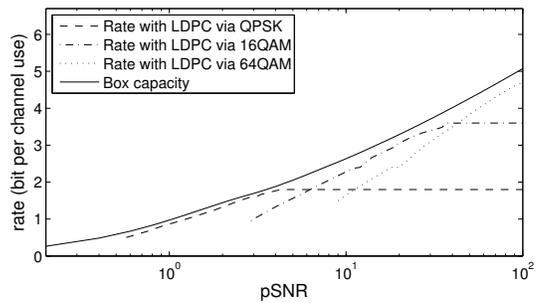
Fig. 6. Achievable rates with QPSK, 16QAM, and 64QAM compared with capacity under box constraint.
