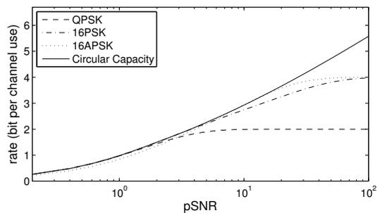
Fig. 4. Achievable rates with QPSK, 16PSK, and 16APSK compared with capacity under circular constraint.
