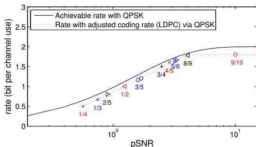
Fig. 5. Rates with adjusted coding rate LDPC via QPSK versus  $\text{pSNR}$ .
