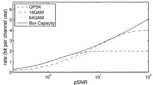
Fig. 3. Achievable rates with QPSK, 16QAM, and 64QAM compared with capacity under box constraint.
