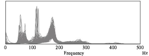
(b) 80 spectrums of deteriorated regulators
