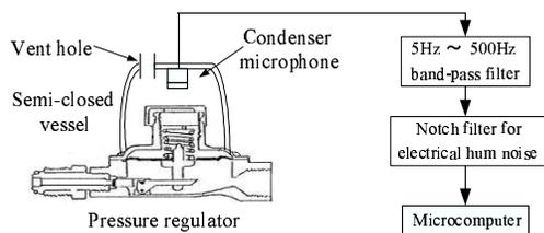
**Fig. 3.** Proposed system for early fault diagnosis of the pressure regulator
