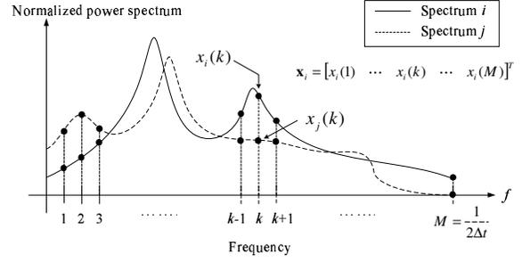
**Fig. 5.** Discretized frequency spectrum for constitution of the feature vector
