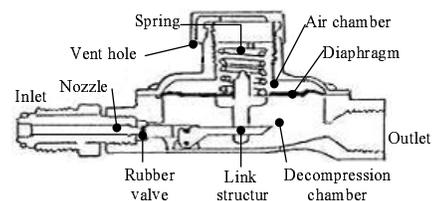
Fig. 2. LP gas single-stage pressure regulator
