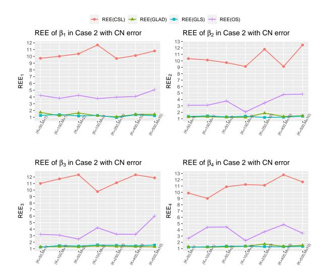
Figure 4: Relative estimation efficiency  $REE_j(OS)$ ,  $REE_j(CSL)$ ,  $REE_j(GLAD)$  and  $REE_j(GLS)$ ,  $j=1,\cdots,4$  versus number of machines K and sample size M under Case 2 with contaminated normal random error.
