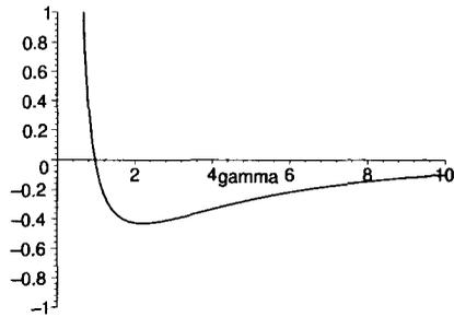
Fig. 6. Relative approximation error  $\frac{1-p_{EA}(\gamma, h)}{1-p(\gamma, h)} - 1$  made using  $p_{EA}$  instead of the exact  $p$  for Example 3.3.
