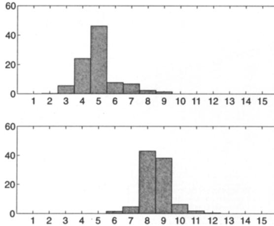
Fig. 5. The histogram for the shrinkage order associated with the sample streams at times  $t = 50$  (top) and  $t = 100$  (bottom) for  $E_b/N_0 = 15$  dB. The fading process is composed of two equal-length parts: the normalized Doppler shift is  $f_d T = 0.005$  in the first part and  $f_d T = 0.01$  in the second part. The result is the average over 100 simulations.
