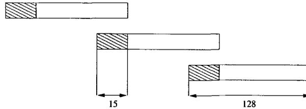
Fig. 2. The frame structure for the nonparametric SMC receivers. The block size is 128, and the adjacent blocks overlap by 15 symbols.
