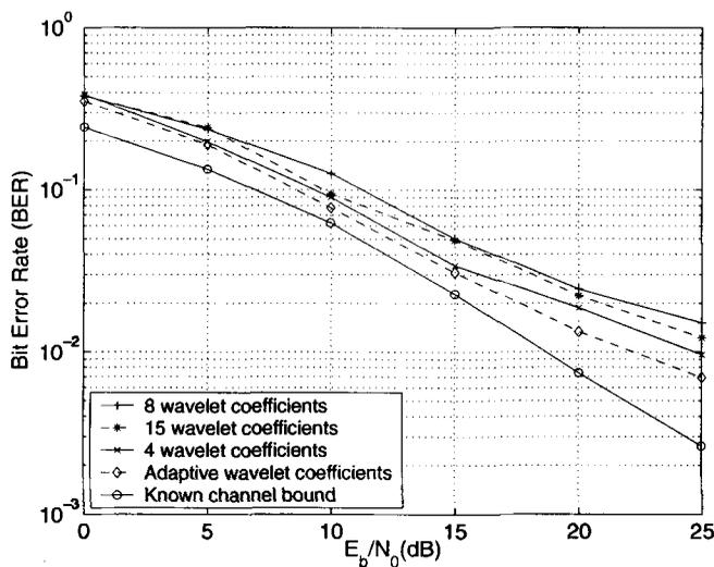
Fig. 7. The BER performance of the blind adaptive receiver. The channel is flat-fading under time varying Dopplers.
