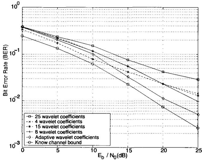
Fig. 3. The BER performance of the SMC receivers. The channel is flat-fading with  $f_d T = 0.005$ . The delayed-weight method is used with  $\delta = 6$ .
