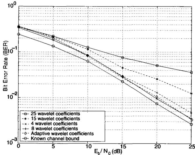
Fig. 4. The BER performance of the SMC receivers. The channel is flat-fading with  $f_d T = 0.01$ . The delayed-weight method is used with  $\delta = 6$ .
