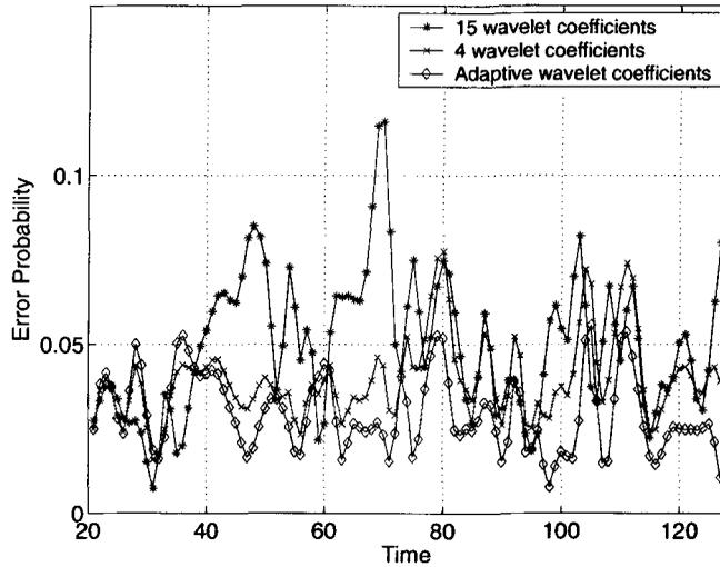
Fig. 6. The BER performance of the blind adaptive receiver at different time points for SNR = 15. The channel is flat-fading under time-varying Dopplers.
