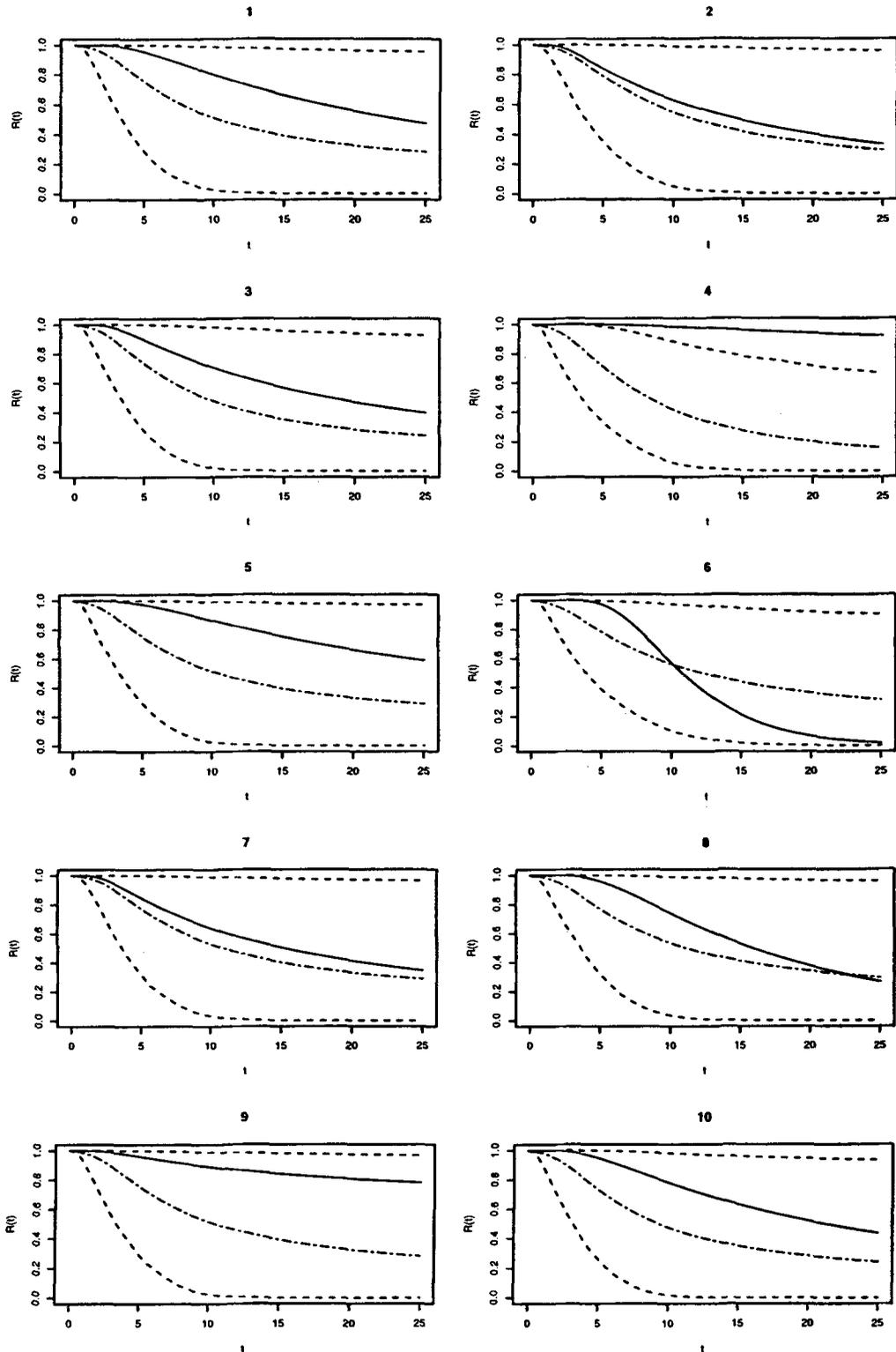
Fig. 5. Cross validated reliability prediction in the exchangeable model. The solid line is the "true" reliability. The middle dashed line is the predictive mean and the outer dashed lines represent a pointwise 90% prediction band.
