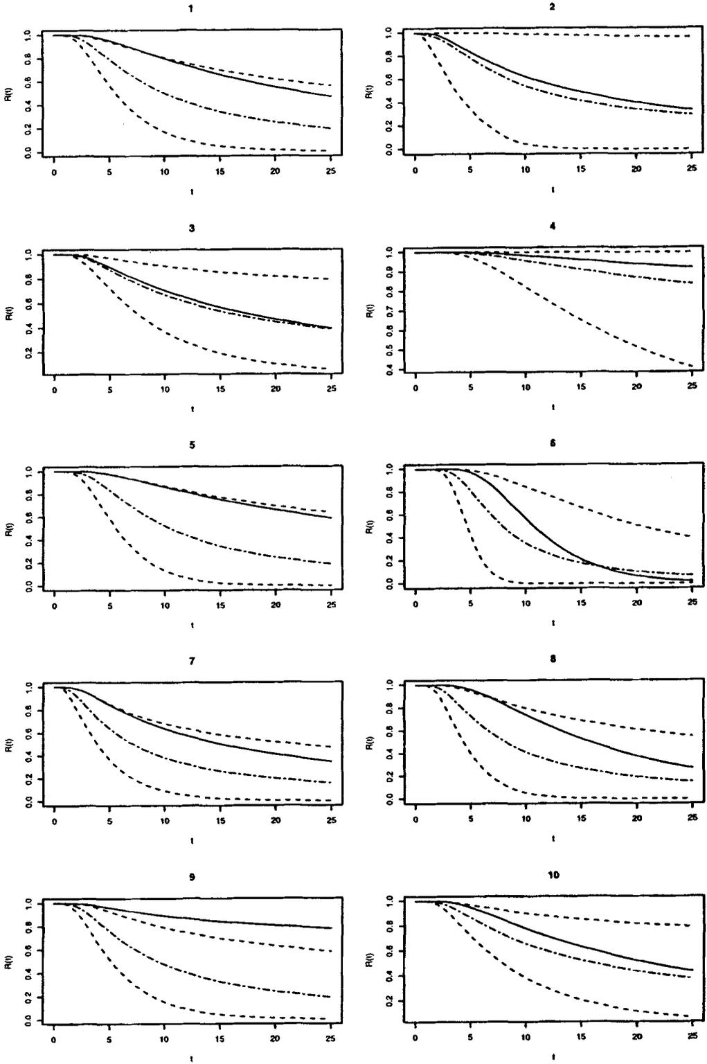
Fig. 4. Reliability estimation in the exchangeable model. The solid line is the "true" reliability. The middle dashed line is the posterior mean and the outer dashed lines represent a pointwise 90% credible band.
