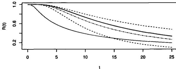
Fig. 2. Reliability estimation. The thick solid line is the “true” reliability. The thin solid line is the mle. The middle dashed line is the posterior mean and the outer dashed lines represent a pointwise 90% credible band.
