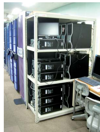
Figure 2: Data assimilation research is carried out with a wide variety of the parallel computing systems including the handmade parallel computing system (above) as well as a general-purpose super computer.
