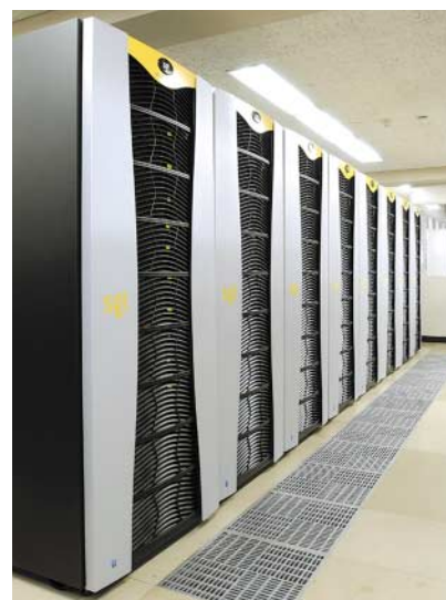
SGI Altix3700 Super Cluster, a parallel computer
