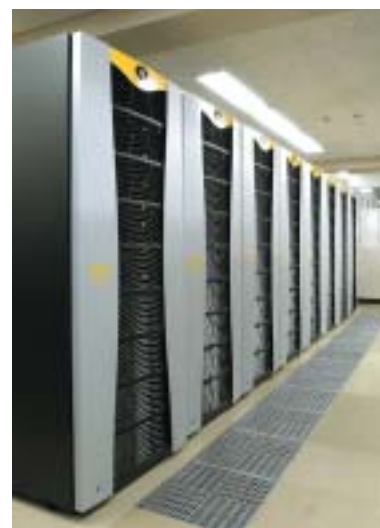
SGI Altix3700 Super Cluster, a parallel computer
