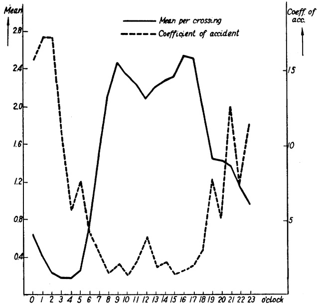
Fig. 7.1. The coefficient of accident and the mean traffic volume in time bands (Sample of size 1000)—Passenger cars.
